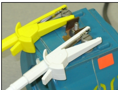
Connect to secondary (white=dot)
